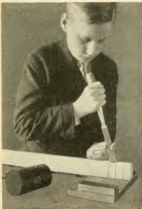
Fig. 20. Method for Holding Chisel in Mortising.
